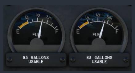
NOTE: Conventional fuel sender units in aircraft are notoriously sensitive to lateral G-force, and how level the aircraft is sitting on the ground. The fuel quantity gauges may appear to indicate incorrectly, as a result, though this is accurate to the real aircraft. Given that this aircraft is also capable of random fuel leaks, fuel levels should be checked prior to takeoff, just as in the real aircraft, when any potential discrepancy exists.
