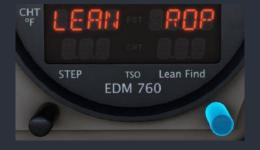
Both methods of leaning begin by "pre-leaning" the engine to approximately 50°F (28°C) EGT rich of peak on any cylinder. After waiting for temperatures to stabilize, begin leaning the engine. When a dot begins flashing above one of the cylinder columns to indicate the hottest cylinder, Lean Find mode is now armed, and an approximately 15°F (8°C) increase of average EGT has been observed.
