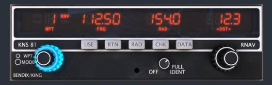
NOTE: VOR modes of operation WILL NOT provide CDI or DME information relative to the active waypoint. They are for operation as a conventional navigation radio with reference to existing VOR stations, in either angular or linear course deviation mode.
