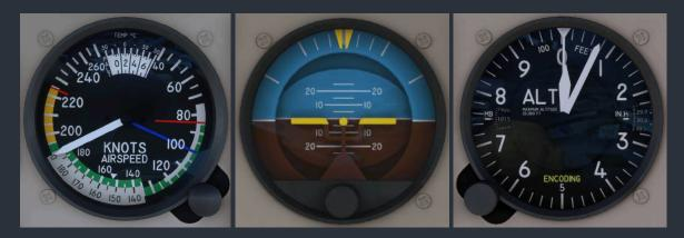
NOTE: This attitude indicator is equipped with Black Square's highly accurate gyroscope dynamics simulation. Users can experience the multitude of gyroscope dynamics and failures inherent to the operation of these instruments. For more information on Black Square's gyroscope simulation, see the "Gyroscope Physics Simulation" section of this manual.
