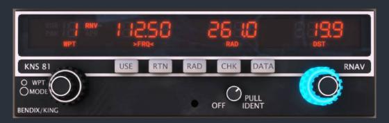
3. Once our desired frequency has been set we will use the "DATA" push button to page through the three required pieces of data in this data channel in the order "FREQ", "RAD", and "DST". Press the "DATA" button once, and then enter the radial 154.0, again with the dual concentric rotary knobs. Should your desired radial include a decimal component, the inner rotary knob can be pulled and rotated for decimal entry.
