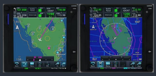
It is now possible to manually switch between PMS and TDS products while the aircraft is loaded. Click on the blue memory card on the left of the unit's bezel.
